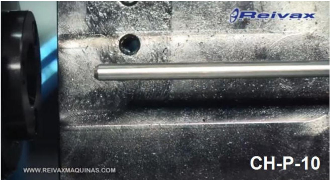
Chamfering head for chamfering the end of the rod.
